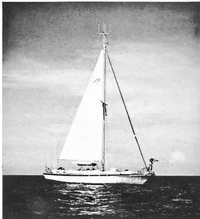
Figure 6. Tagging and tracking arrangements on a Morgan 41 sloop. A platform was constructed on the bow ahead of the mast stay for unobstructed tagging, and the Adcock ADF antennas were mounted at the top of the mast. (Photo by Moore)
